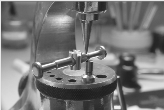
Assembling vernier for azimuth
